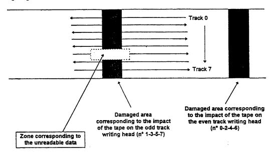
The UFDR writes blocks of 784 bits of data (corresponding to 1 second). Each block is separated by an IRG (Inter Record Gap). The last second written on the tape is followed by a blank area corresponding to the erasure of the track by the erasure head of the recorder. In consequence, the following diagram shows the structure of the zone to be examined:
