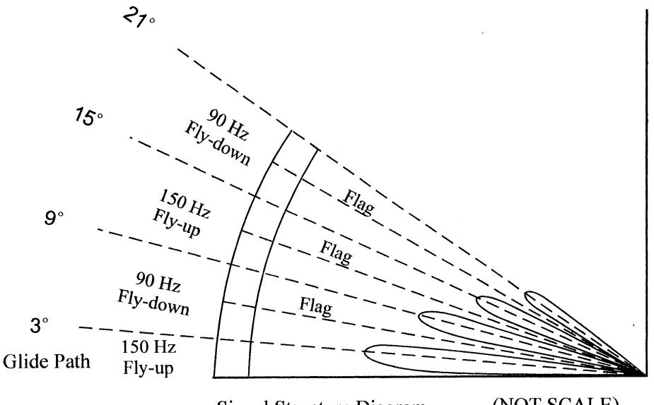
Signal Structure Diagram
