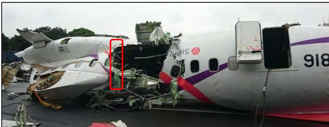
Figure 1.3-3 A broken area on the right hand side fuselage located at frame 28-28A area
