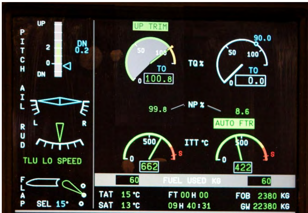
Figure 1.6-3 Simulated EWD display of ENG 2 autofeathering at takeoff
