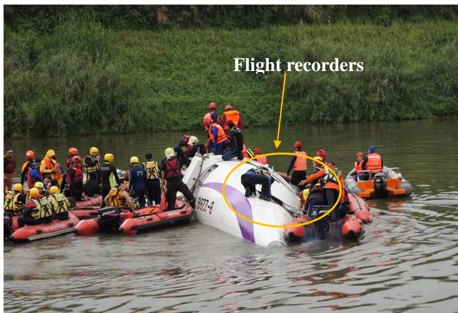
Figure 1.11-1 Flight recorders were recovered by ASC investigators
