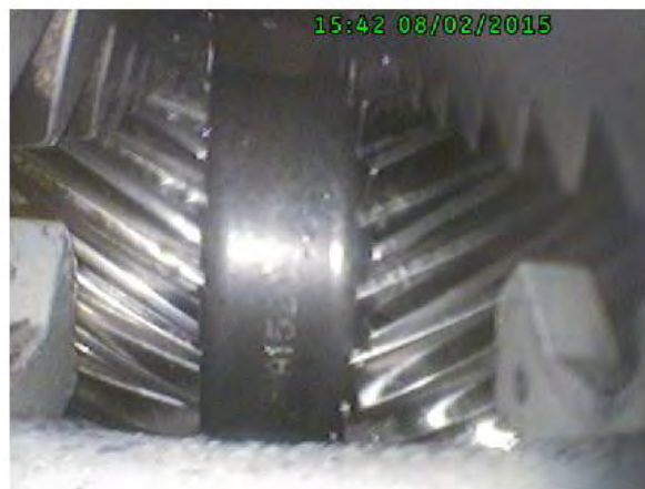
Photo No. 16 Reduction gearbox helical input gearshaft and helical gear.
