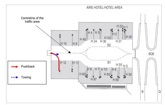
On the day of the accident, the ground was icy in places. The driver stated that the airplane was improperly aligned after pushback because of the slippery ground and that he had tried to re-align the aircraft by pulling it forward.
