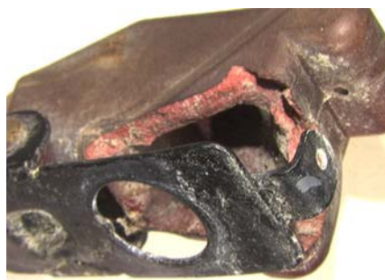
Figure 62: Bottom view of switch guard damage.
