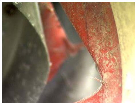
Figure 231: Outer diaphragm damage.
