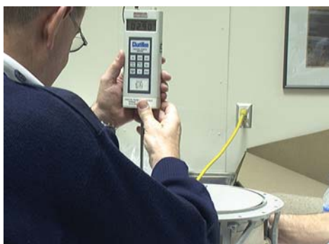
Figure 268 : Comparison unit*, door B tension, 2.90 pounds (opening force from center edge of door)
