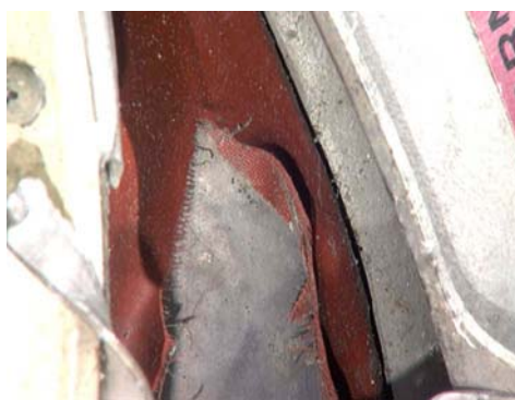
Figure 233: Outer diaphragm, close-up of tear origin.
