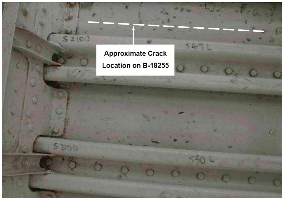
Figure 1.6-12 A B747-200 aircraft bilge area with the CIC and dust removed
