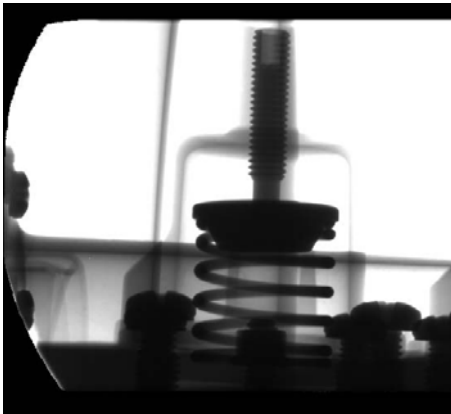
Figure 244: Integral sense control, adjustment spring.
