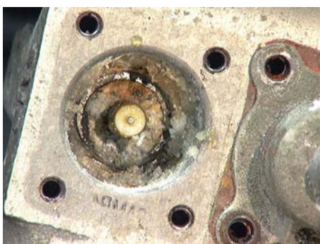
Figure 251: Close-up of salt deposits inside housing bore.
