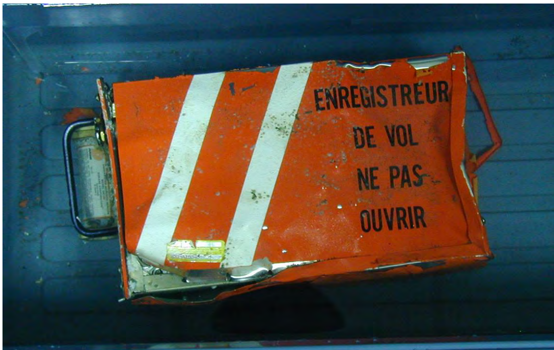
Figure 1.11-1 Damaged CVR in the water cooler
