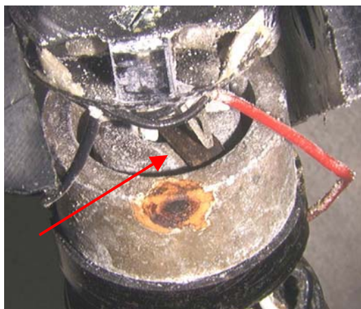
Figure 17: LEFT, OUTFLOW VALVES Position Indicator witness mark
