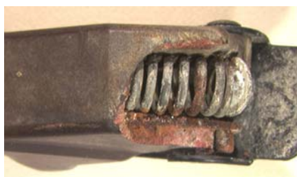
Figure 61: Top view of switch guard damage.
