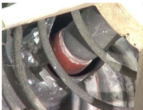
Figure 235: Center diaphragm, HS P/N 727401-1 appears to be intact and the bond portion can be seen; looks normal.
