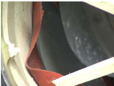
Figure 230: Outer diaphragm damage.
