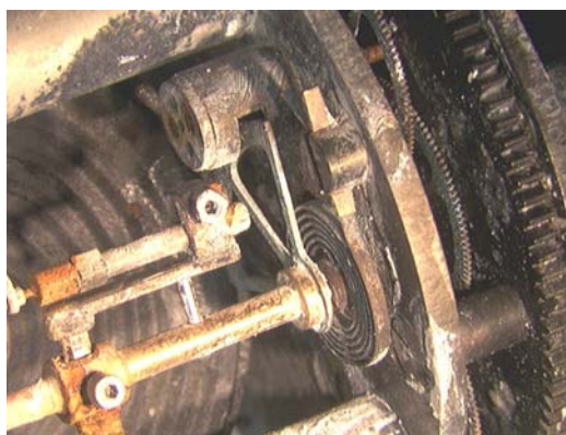
Figure 46: Cabin Altimeter Indicator, bellows, visible damage
