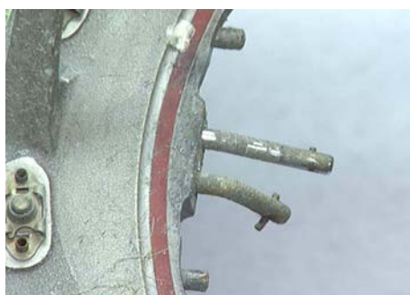
Figure 106: Aft hinge & stop pins (looking from inside to outside).
