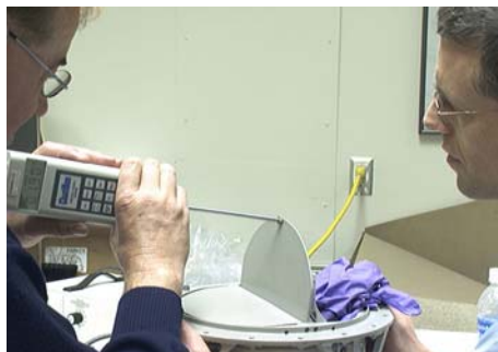
Figure 269: Comparison unit*, door A compression (closing), 1.90 pounds (push at center of door to close door).
