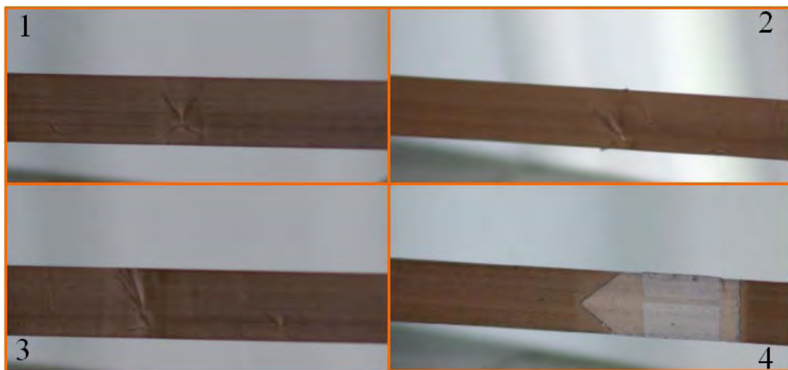
Figure 2.6-1 Damaged and spliced tape areas
