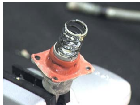
Figure 166: Diaphragm appears to be intact.
