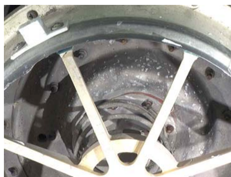
Figure 155: Gate return spring, showing unseated spring.
