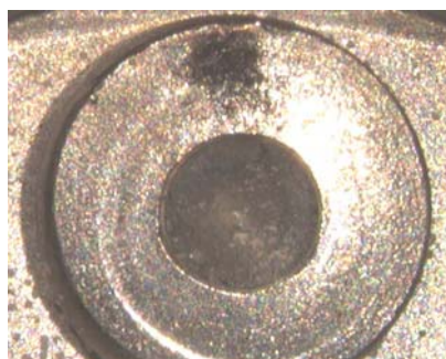
Figure 56: Movable contact of oxygen control switch " ON " position.
