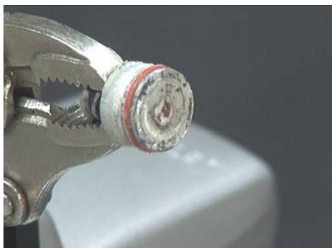
Figure 253: Plug HS P/N 719280-1 and seal, seal looks normal and uncut.
