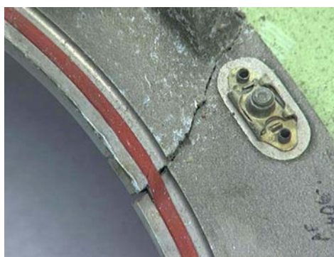
Figure 98: One slight cut adjacent to housing fracture.
