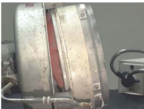
Figure 149: Offset angle between valve housing and gate.
