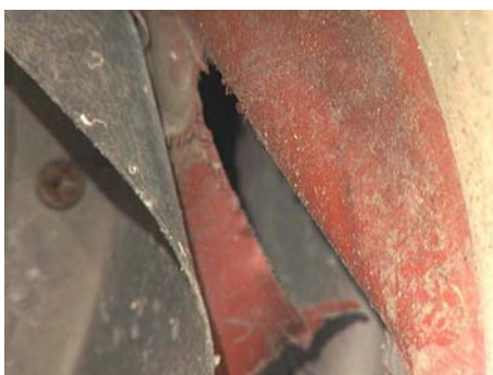
Figure 228: Outer diaphragm, approximately 60% of circumference is torn.
