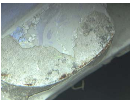
Figure 202: Close-up of figure #200, paint chipped.
