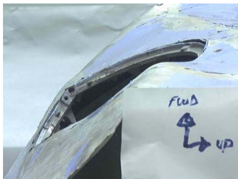
Figure 183: Skin distortion at valve mounting location.
