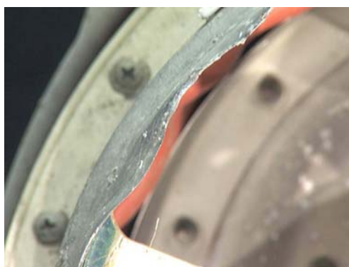
Figure 139: Close-up of knife-edge damage.
