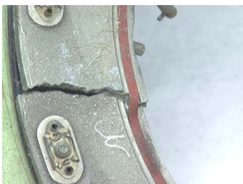
Figure 97: Non-metallic washer (gate seal) - continuous ring.
