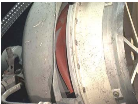
Figure 148: Diaphragm, circumferential tear.
