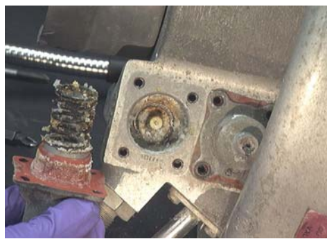
Figure 250: Showing remote ambient sensor removed.
