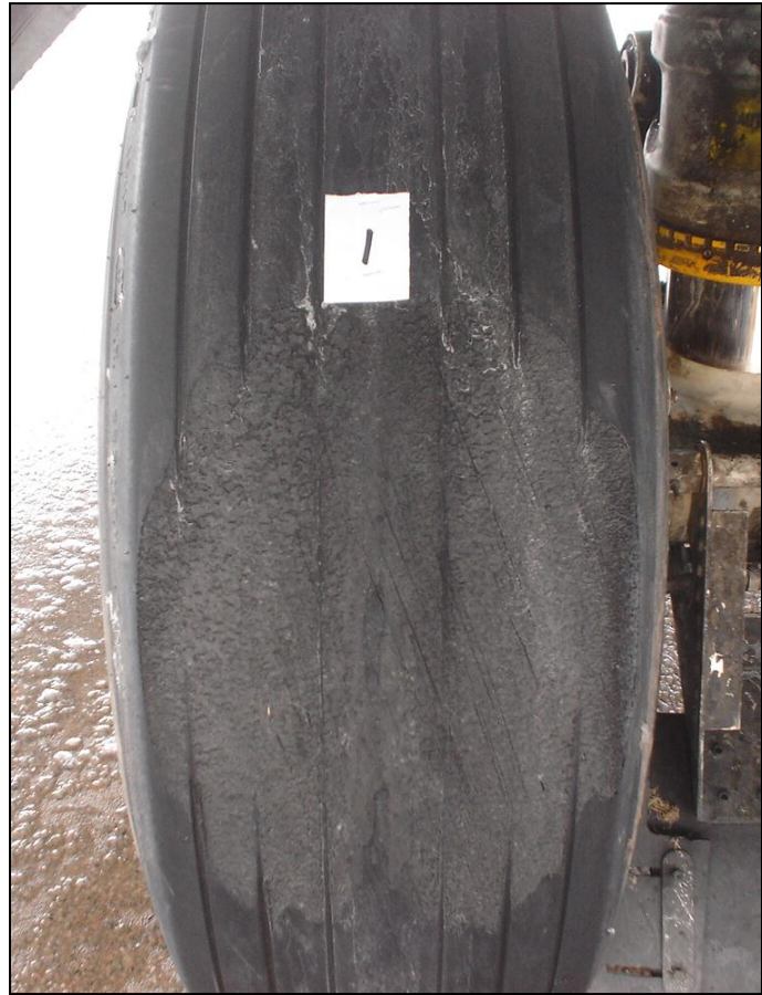
Photo 3. Reverted Rubber Occurrence Aircraft Tire
