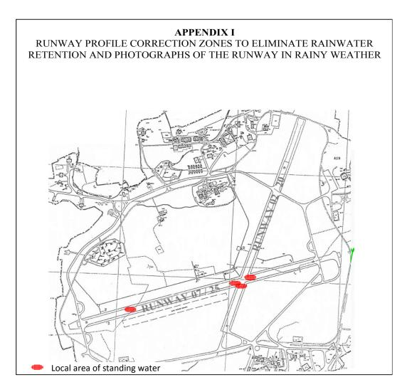
After the accident, two fire trucks poured water on the south side of the runway over the last 1,200 m. Water retention zones were found on certain sections<sup>(16)</sup>.
