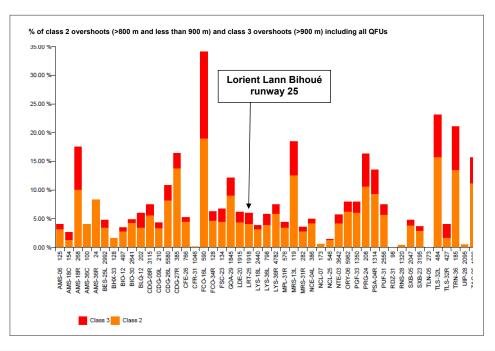
At the request of the BEA, the airline forwarded the graph for overshoots by CRJ-700 on runways where the LDA is less than 2,400 m. It shows that 551 out of 1,680 landings occurred more than 650 m from the threshold, i.e. 32.8% of the landings (see Appendix 9). In this classification, it can be seen that the largest number of overshoots occurred at Lorient Lann Bihoué.
