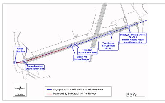
The positioning of the thrust levers to IDLE and touchdown of the main landing gear occurred respectively at 330 and 1.130 m from the threshold of runway 25.
