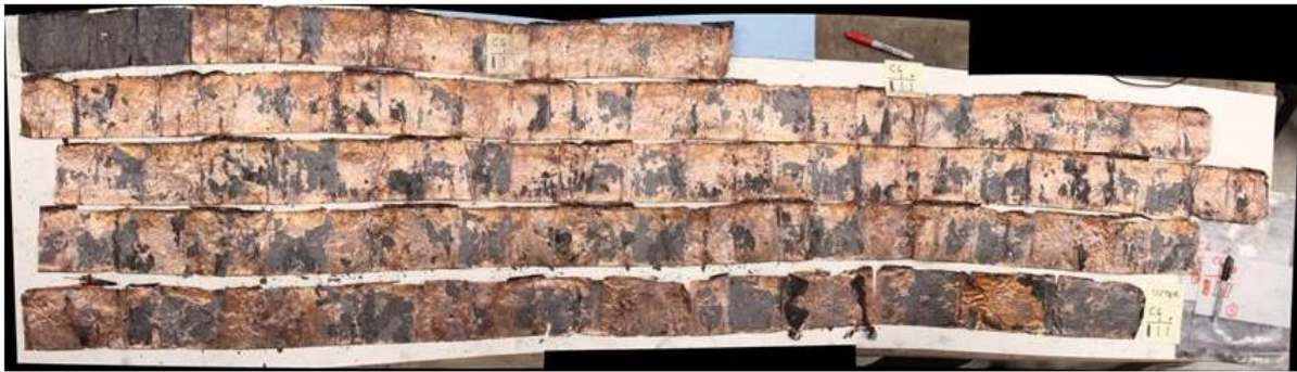
Figure 14. Cell 6 winding closest to cell 5.
