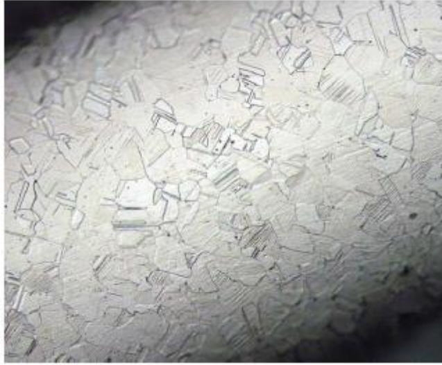
Microstructure of the investigated stainless steel spring, 200X
