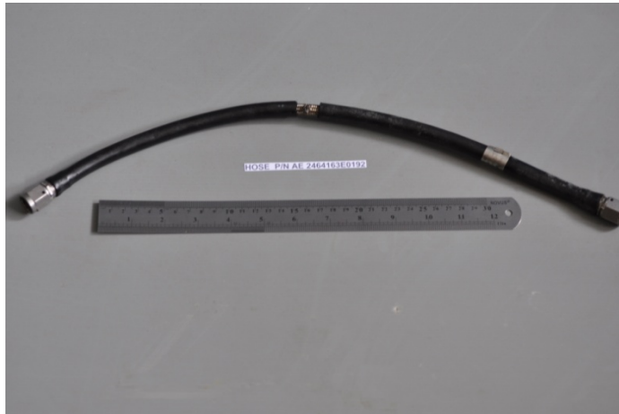
Figure 7: The hose shows damage in the middle
