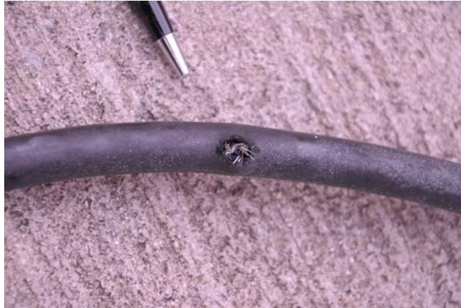
Figure 1: Hydraulic Hose shows burst at middle position
