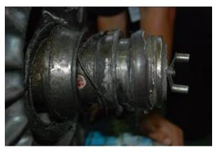
Figure 1: Bearing failures on the axle.
