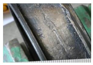
Figure 4: Dull surface on the inner raceway of the outboard bearing. Note the roller impressions indicating false Brinelling due to vibration.
