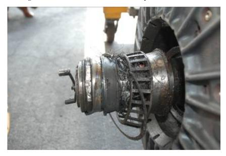
Figure 3: Damaged inner and outer wheel bearing race on number-two axle
