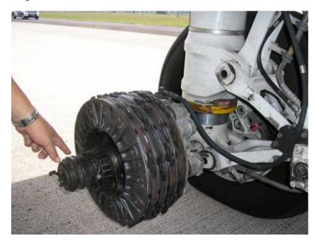
Figure 2: The number-two main wheel separated from its axle
