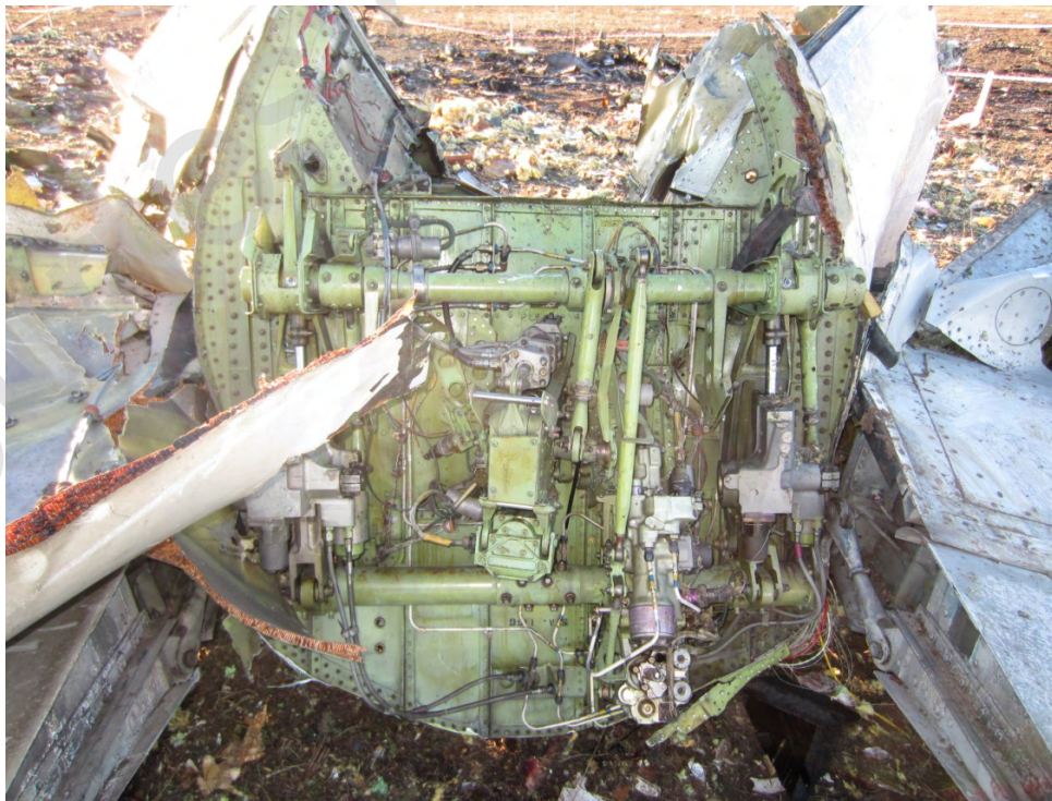
Figure 20 Tail cone fragment
