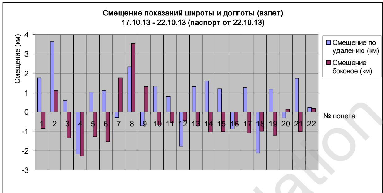
Figure 80 IRS map shift during takeoffs on October 17 to October 22, 2013
