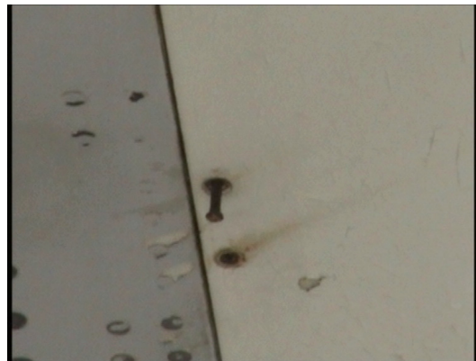
Example of a loose screw on a lower wing panel
