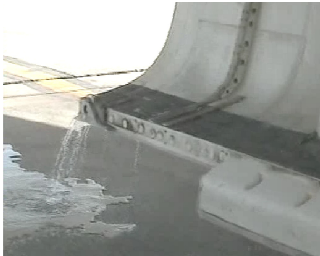
Fuel leak detected on opening a landing gear door
