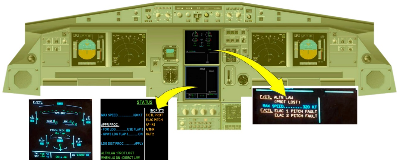
Figure 1. Messages displayed on ECAM on F/CTL ELAC 1 and 2 PITCH FAULT - ECAM F/CTL system page, ECAM status page, ECAM Engine/Warning display
