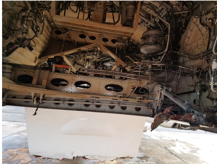
Figure 35 RH landing gear actuator and missing door
