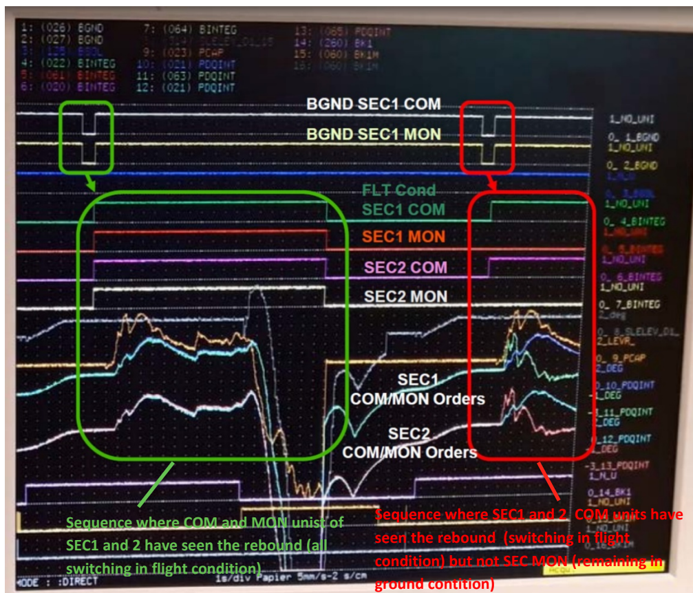
Figure 63 Rebound test with two LGCIUs and SECs. SEC COM and MON seeing ground/flight condition
