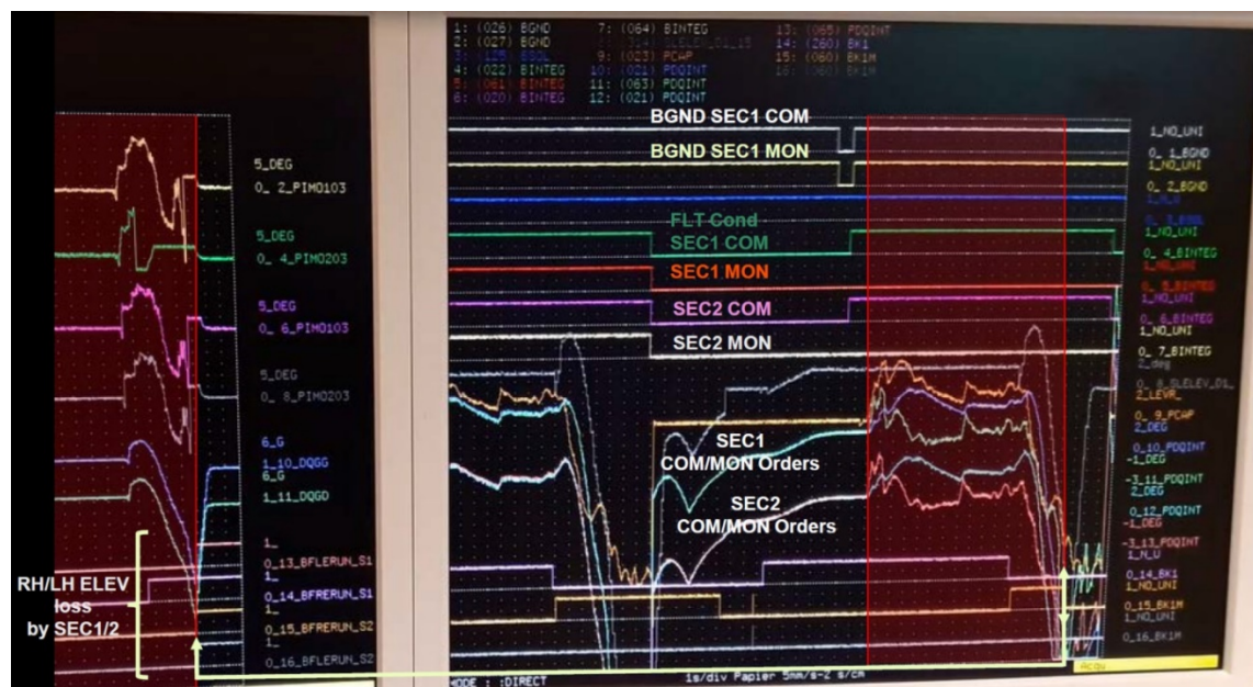
Figure 64 Loss of ELEV control by the two SECs by the discrepancy between SEC COM and MON Ground/Flight condition
