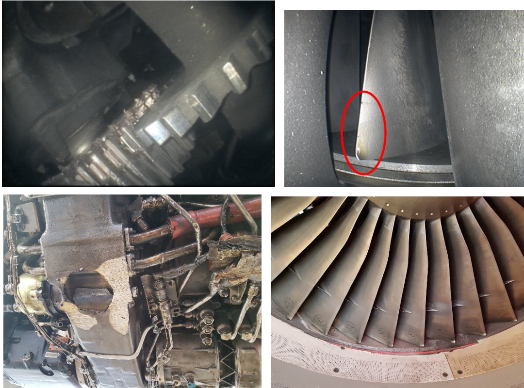
Figure 32 Bound gears in AGB; minor tip curl at compressor stage 4; Perforated AGB case; Fan blade tip curl and scraped lining.
