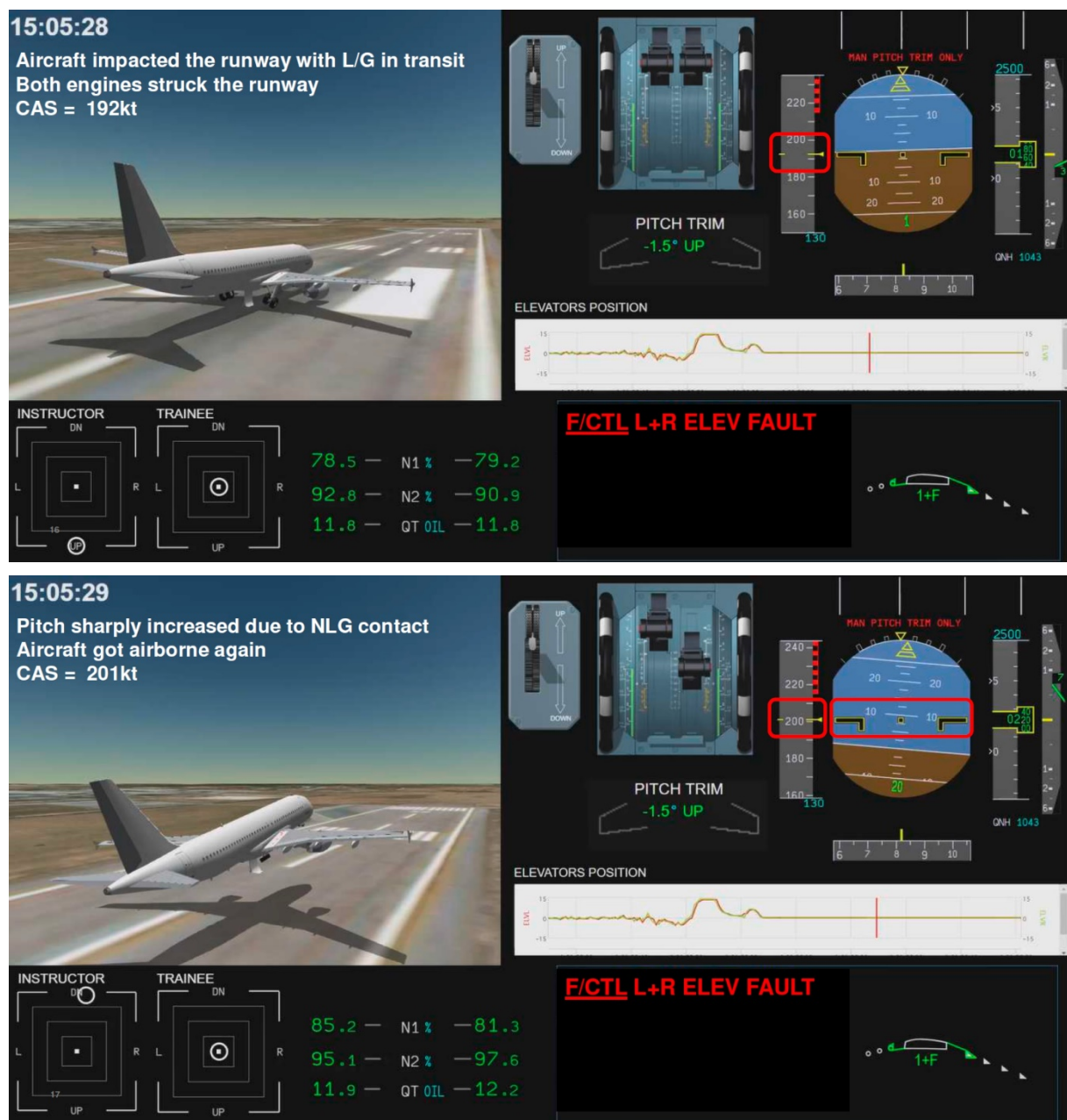
Figure 7. Cockpit inputs and indications at 15:05:28 and 15:05:29
