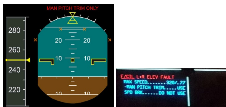
Figure 17 PFD display in PITCH mechanical back-up, ECAM procedures displayed in mechanical backup.
