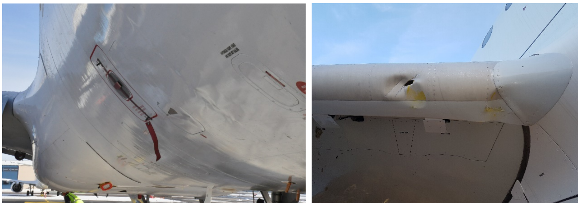
Figure 31 A/C skin wrinkled, fairings damaged by landing lights; slat punctured
