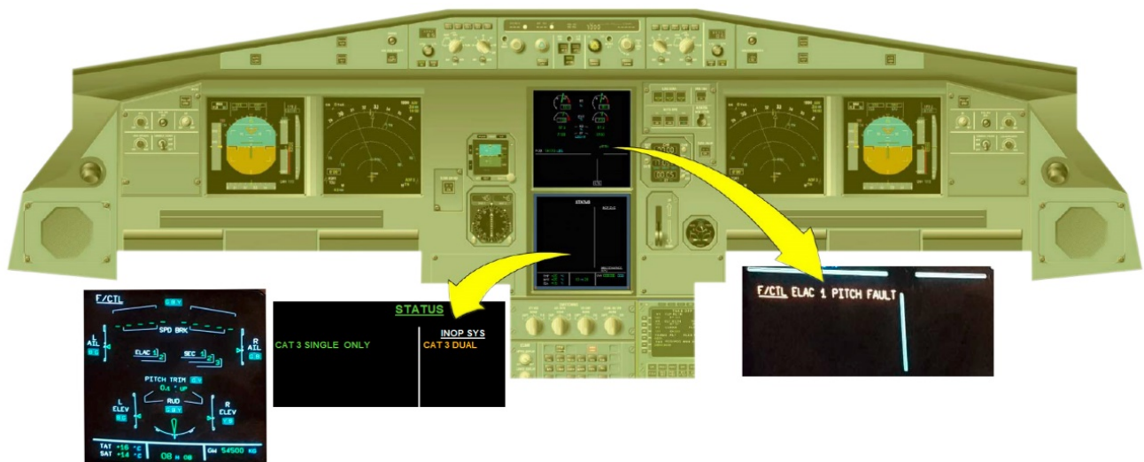
Figure 2. ECAM FC CTL system page, ECAM status page, ECAM Engine/Warning display on the event of ELAC 1 PITCH FAULT
