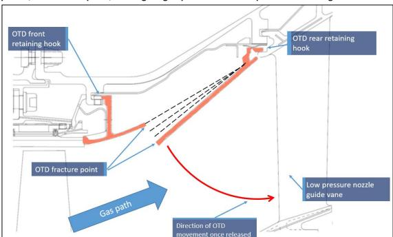
Figure 4: Plan view of the low pressure outer transition duct, front and rear attachment points, the fracture point, the engine gas path and the low pressure nozzle guide vane.
