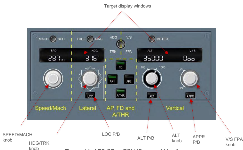
Figure 11. AFS CP or FCU [Source: Airbus]
