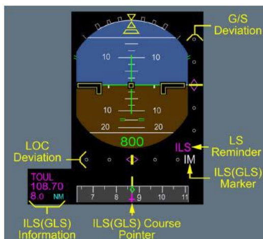
Figure 19. ILS information on PFD [Source: Airbus]
