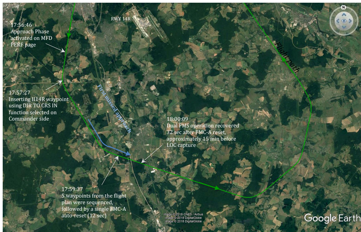
Figure 36. Aircraft trajectory after the go-around and preparation for the second approach
