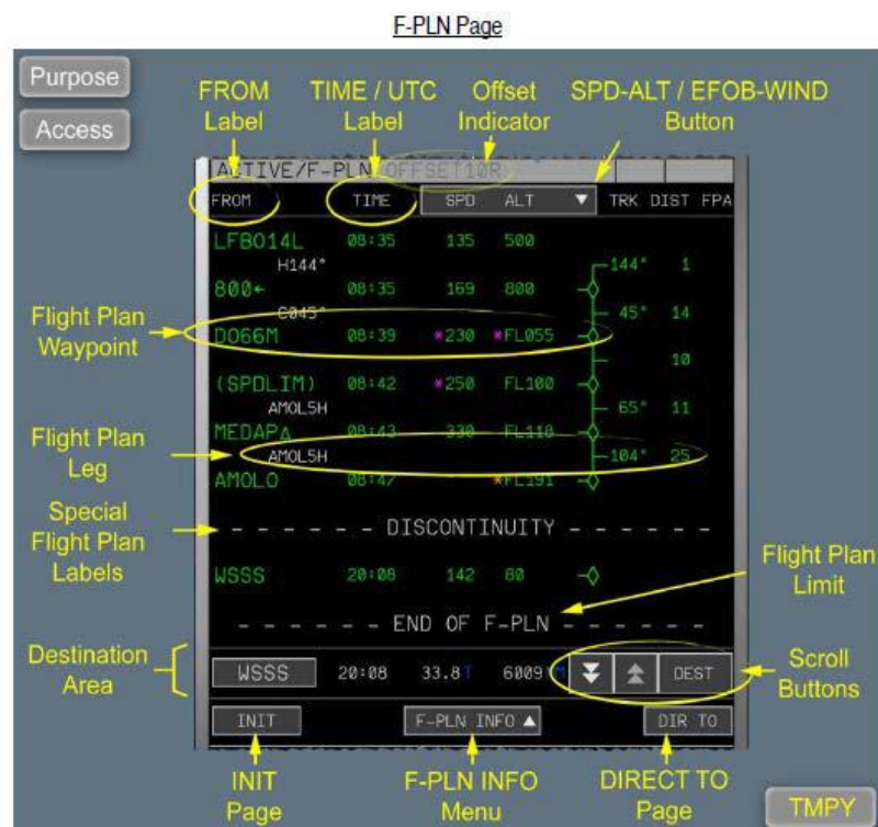
Figure 12 – Example of flight plan page displayed on MFD [Source: Airbus]
