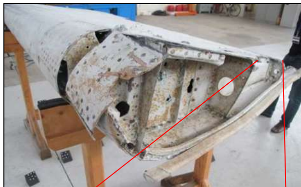
Planche 25 : Elements located aft of the outboard hinge fitting
