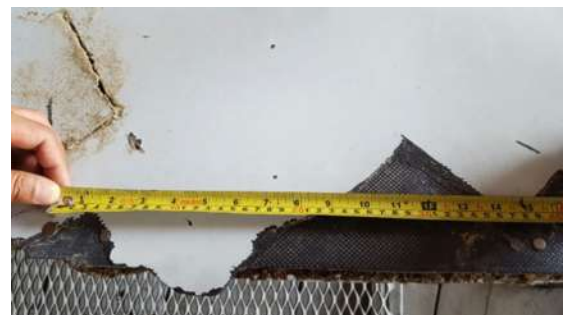
Spacing of fasteners on the debris
