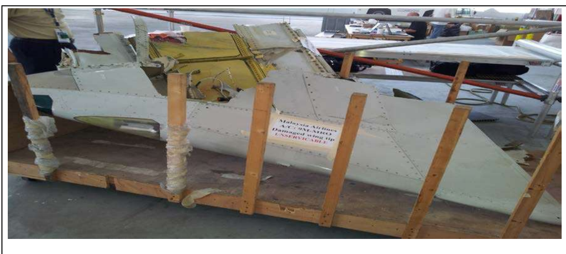
Figure 1.6B - Damaged Wing Tip
