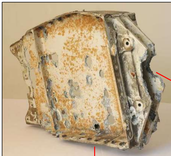
Outboard hinge fitting disassembled
