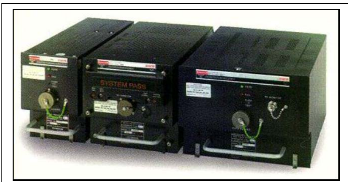
Figure 1.9L - RFU (left), SDU (centre) and HPA (right)
