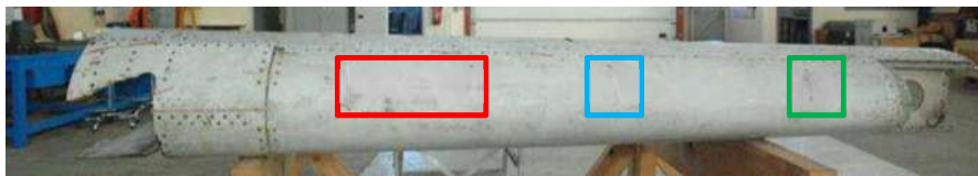
Planche 47 : Impacts on the leading edge
