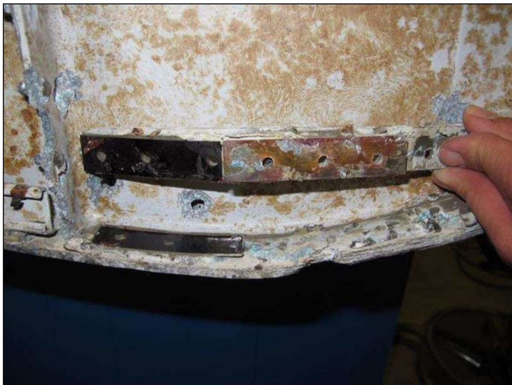
Repair: disassembly of seal retainer
