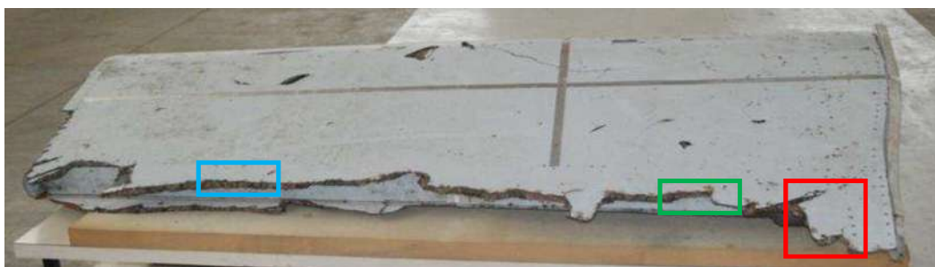
Regular fracture, without protruding fibres
