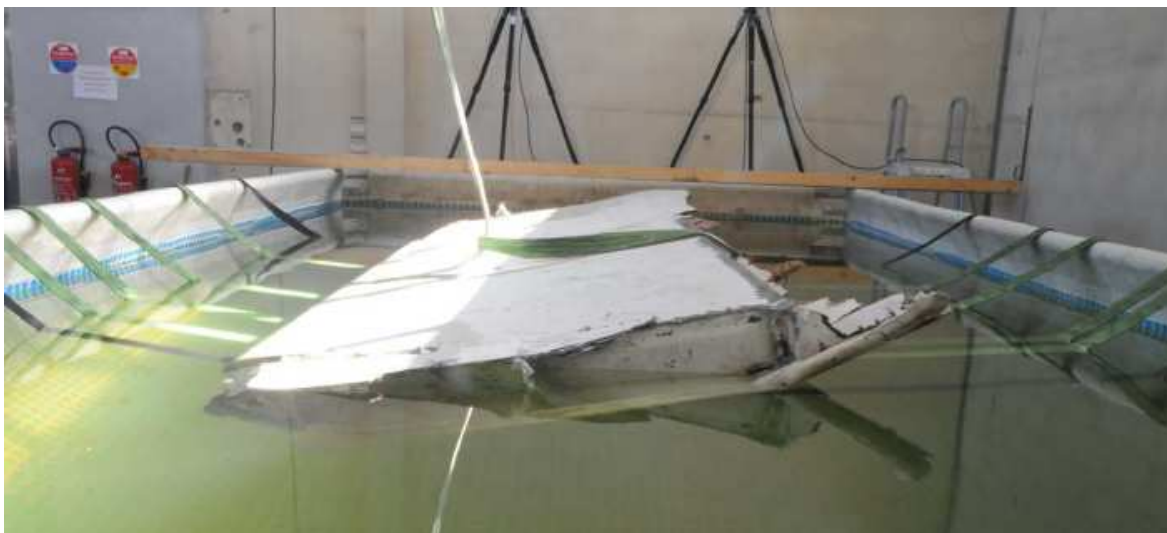
Positioning the flaperon in the pool
