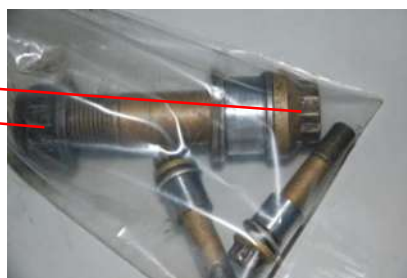
Activator hinge point pin and other attachments
