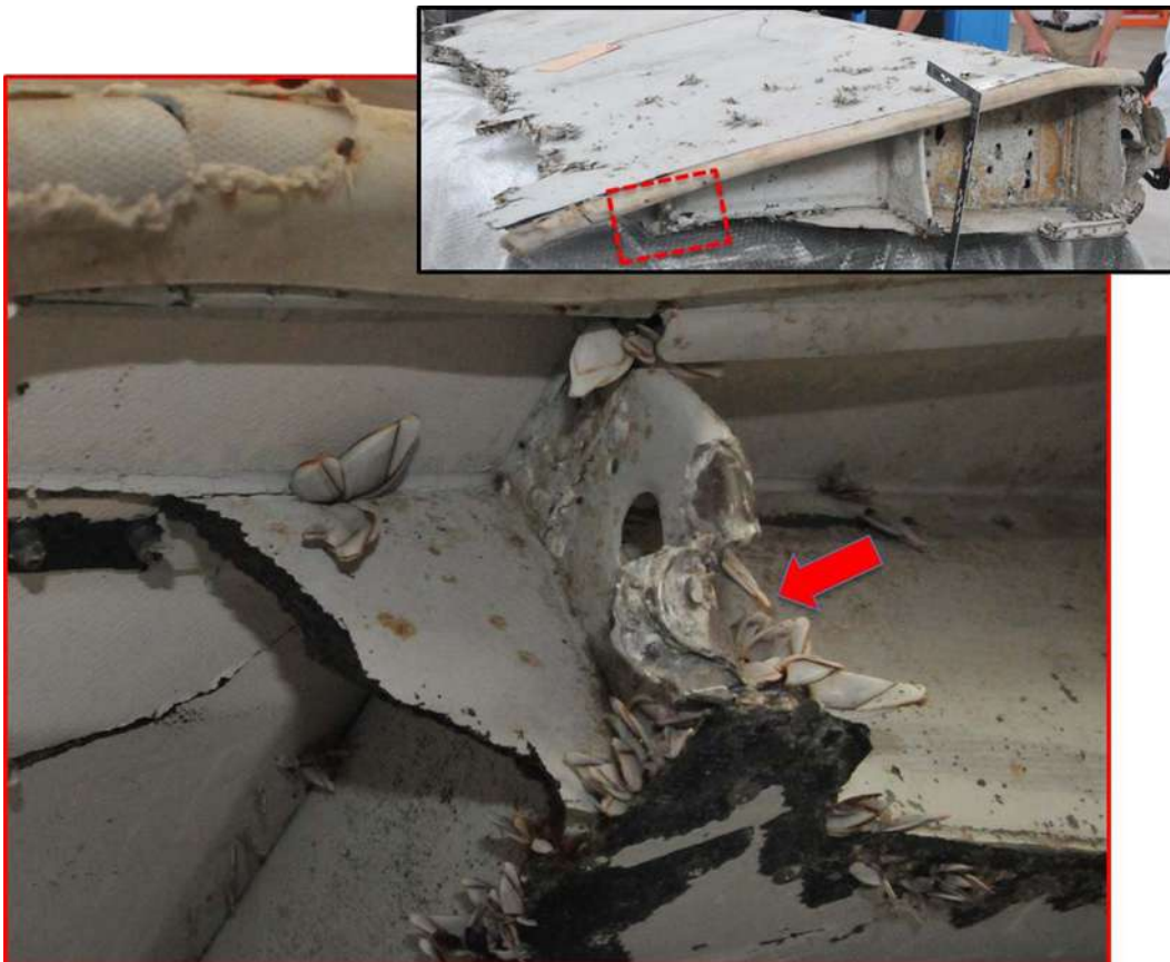
Figure 21: Flaperon, outboard side damage
