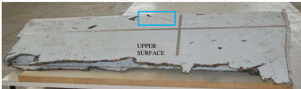
Planche 57 : Upper surface: impact and protruding crack
