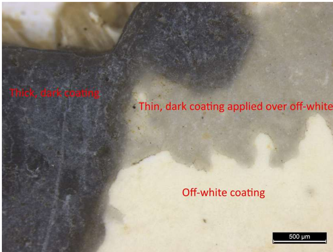
Figure 4: Close-up of applied coatings
