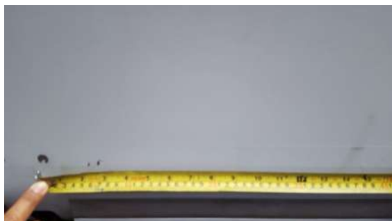
Spacing of fasteners on the aileron on aircraft
