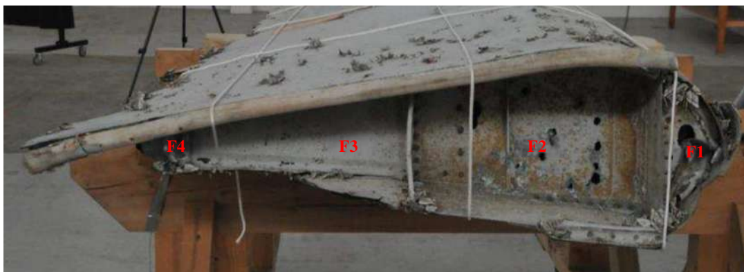
Planche 12 : Detail of zones F on the flaperon
