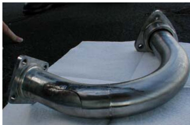
Figure 4 Fuel Pipe Crack & Scratches
