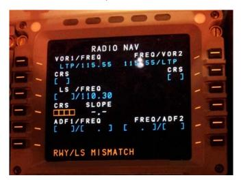
In this example, the font size of the frequency automatically entered by the FMGS (e.g. VOR1 and 2) is by default smaller than that manually entered (e.g. ILS).
