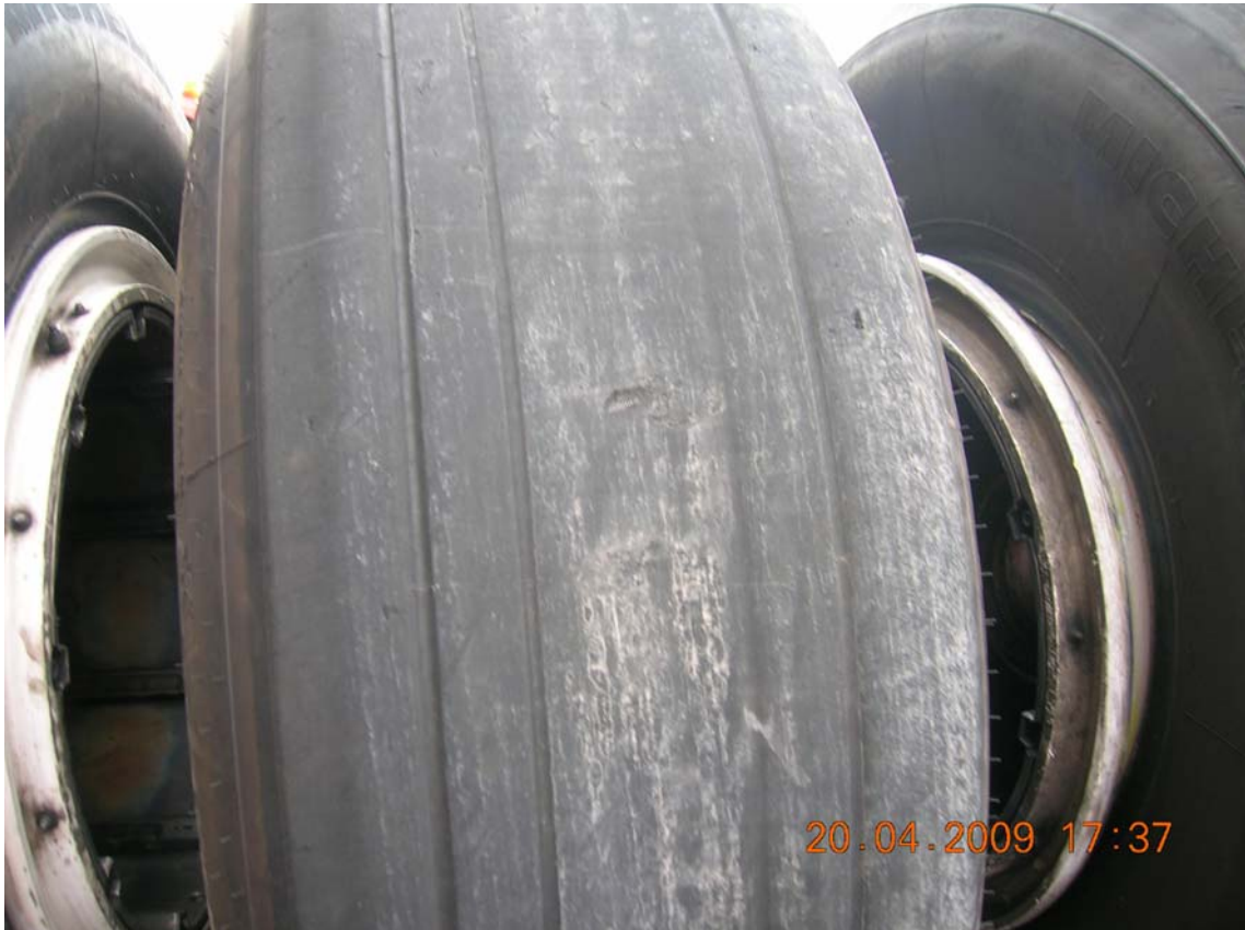
Tyre indicating signs of partial aquaplaning
