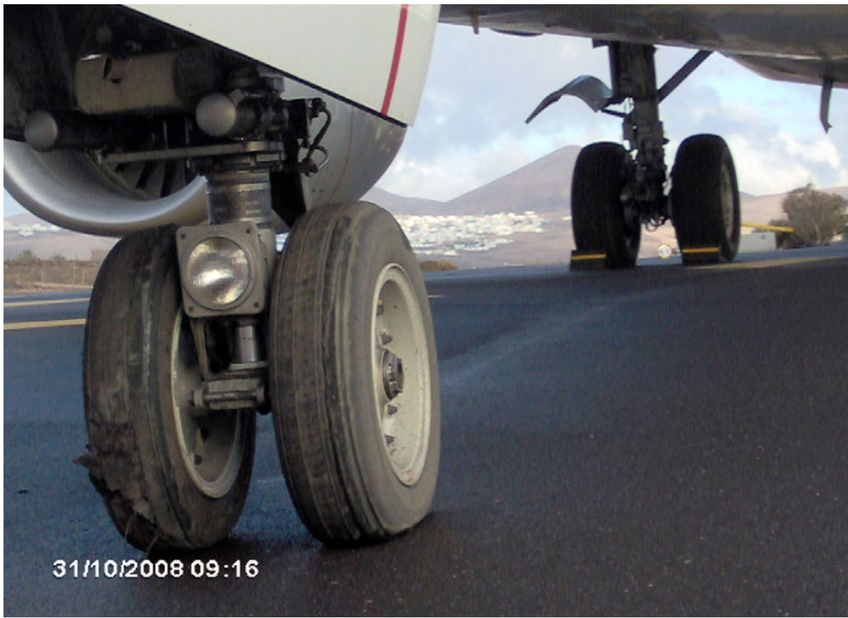
Figure 2. Damage to the nosewheel landing gear
