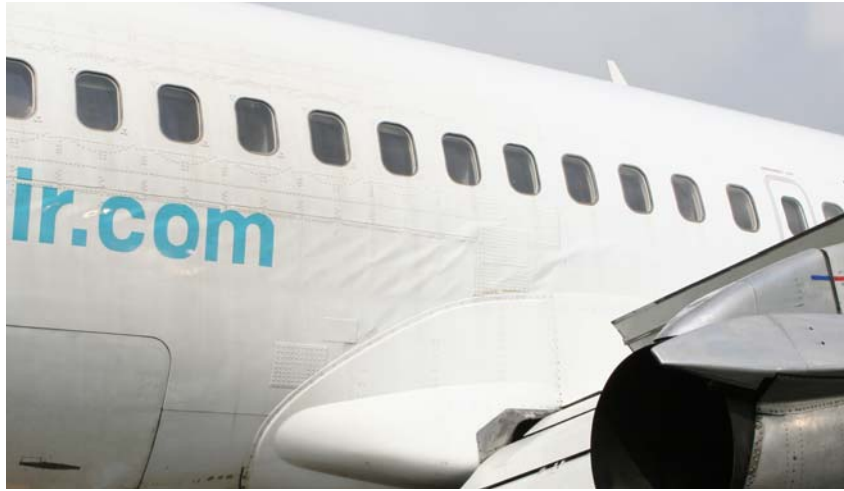
Figure 2: Wrinkling on the right centre fuselage section
