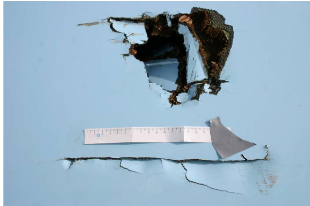
Figure 2. Damage to left engine cowling (close-up view)
