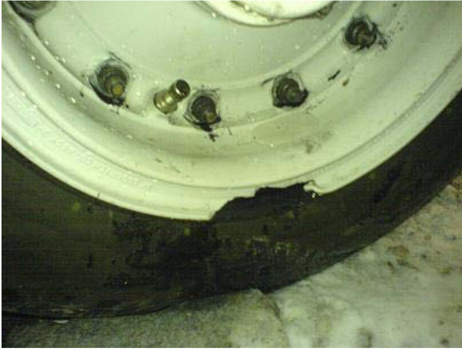
Figure 8: Damage to the nosewheel rim.
