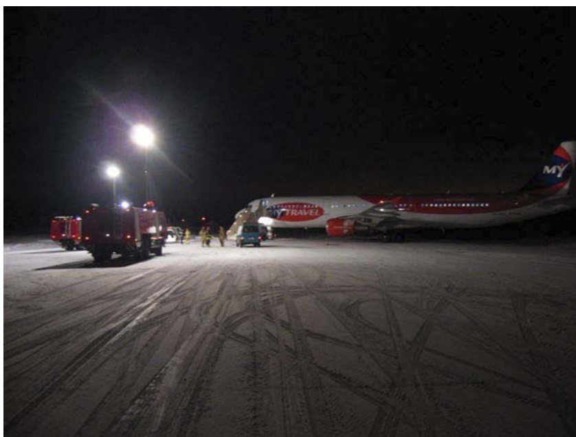
Figure 3: Reflections in frozen moisture in the vehicle tracks indicate a slippery runway.
