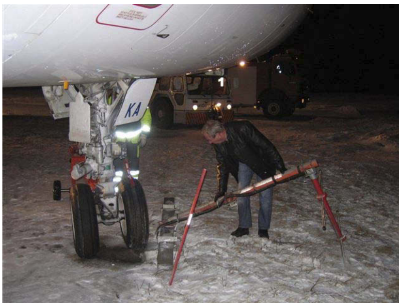
Figure 1: Damaged Localizer Monitoring antenna with concrete base.
