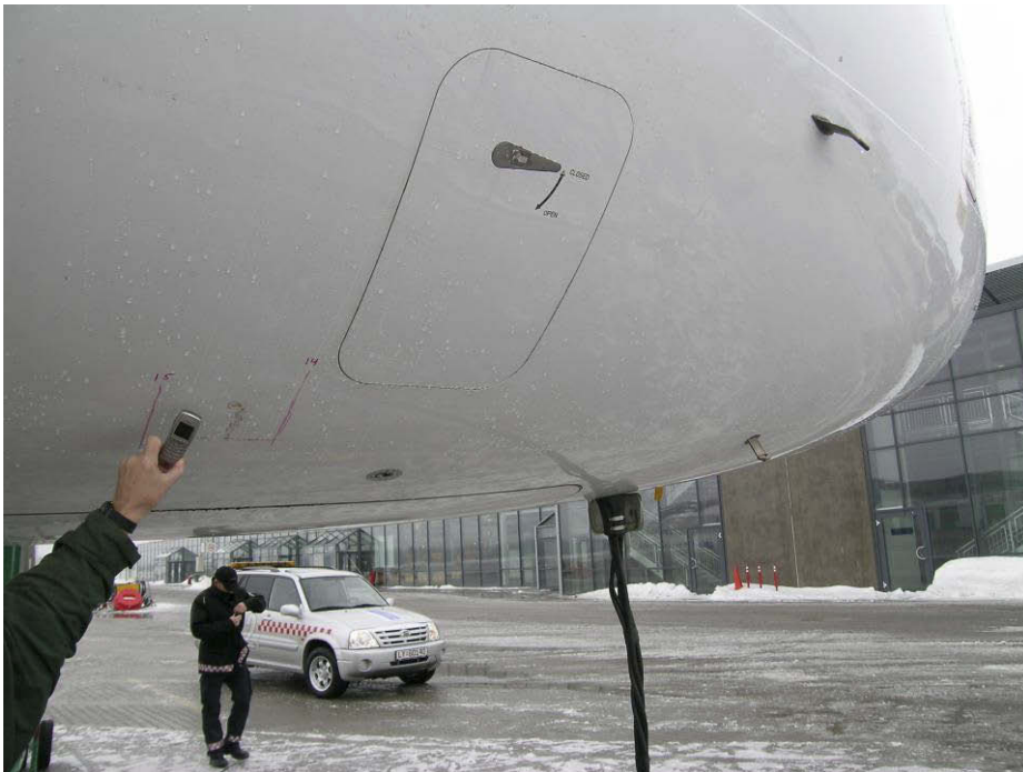
Figure 9: Minor indentation in the fuselage between stations 14 and 15.
