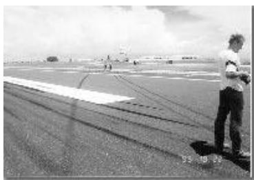
Fig 8. Tyre Marks as aircraft left runway
