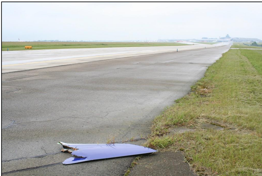
Fig. 2 Scene of the collision and a B737-8BK right wing winglet piece long approx. 1.2 m.
