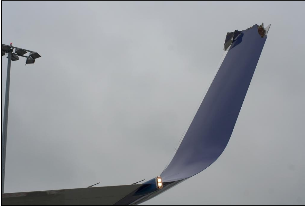
Fig. 5 Damage to B737-8BK right wing winglet.
