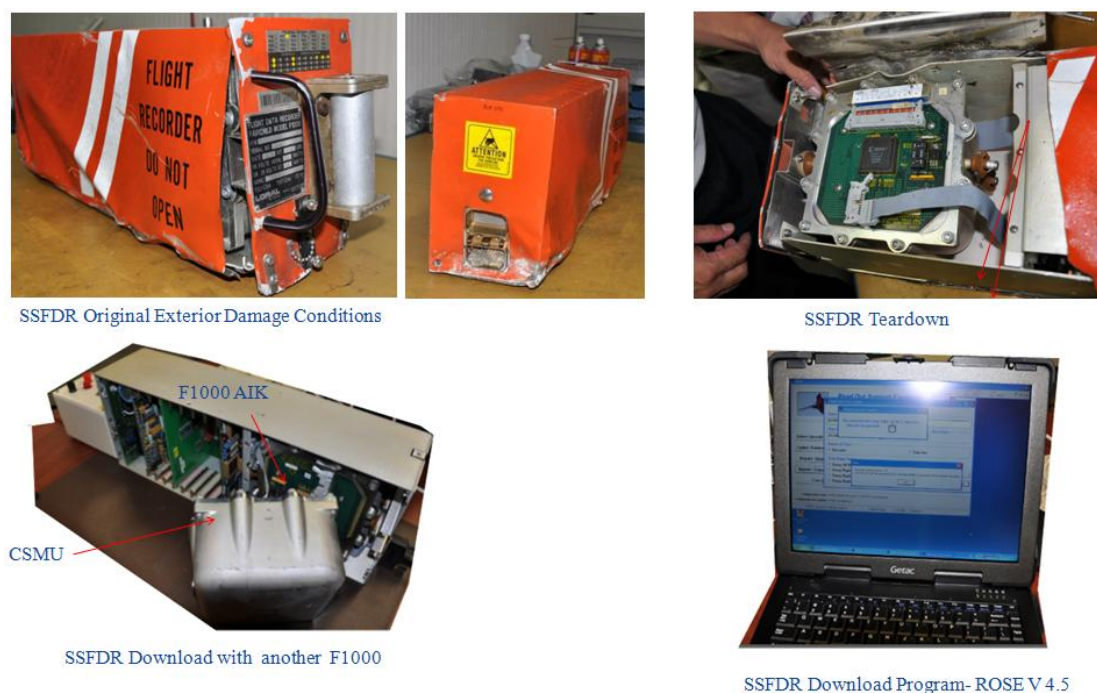
Figure 1.11-2 FDR exterior view, teardown and download process
