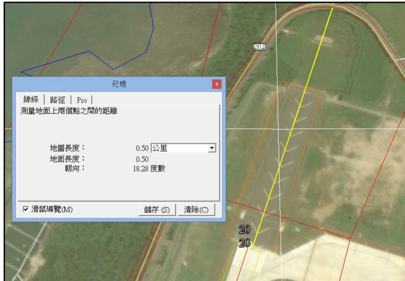
Figure 1.10-3 Available distance measured from Runway 20 (image from Google Earth)
