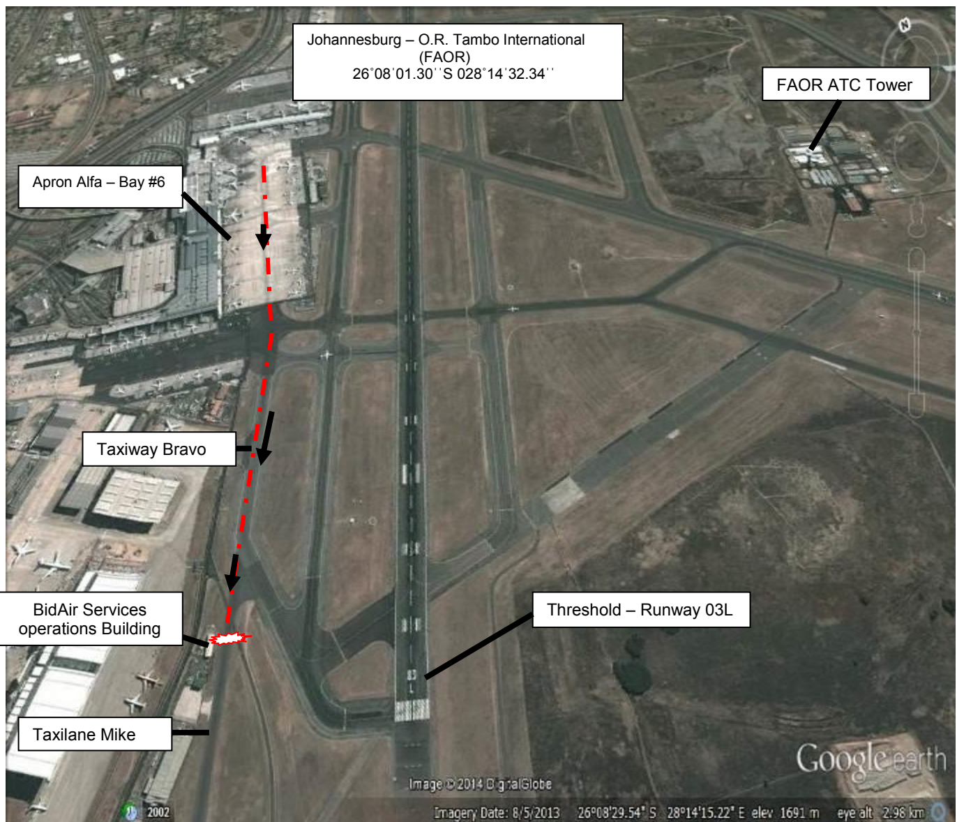
Figure 2 Actual taxi route which the pilots followed before the collision with the Bid Air Services Building
