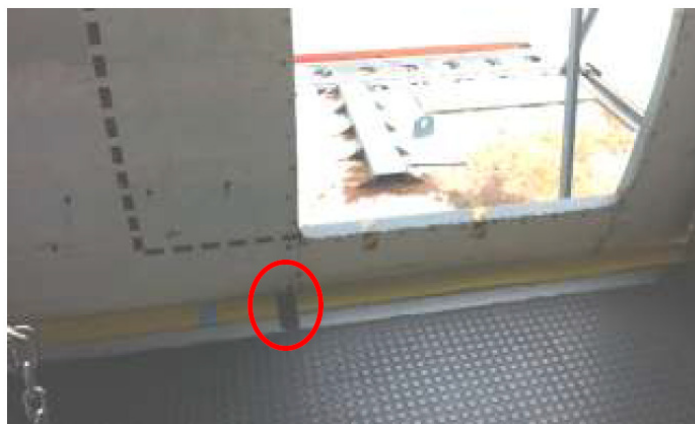
Figure 16: Position of black marking aligned with left edge of front cabin door during normal docking with the mock-up fuselage
