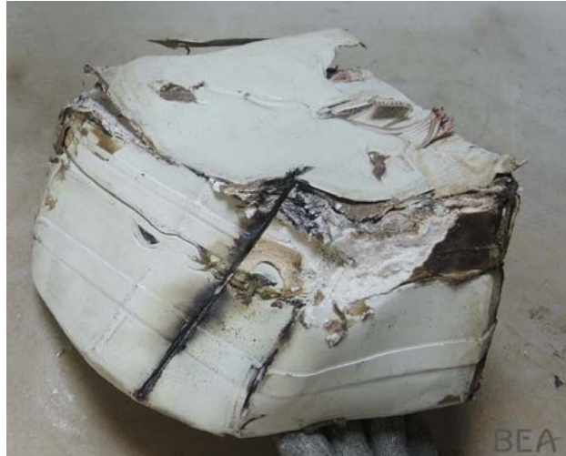
Heat protection of the data media
