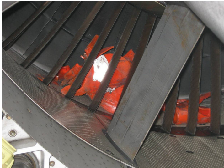
Figure 1: Cone ingested into the No. 2 engine
