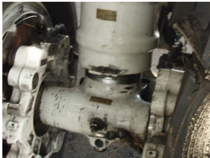
Figure 7: Bottoming mark on right main landing gear
