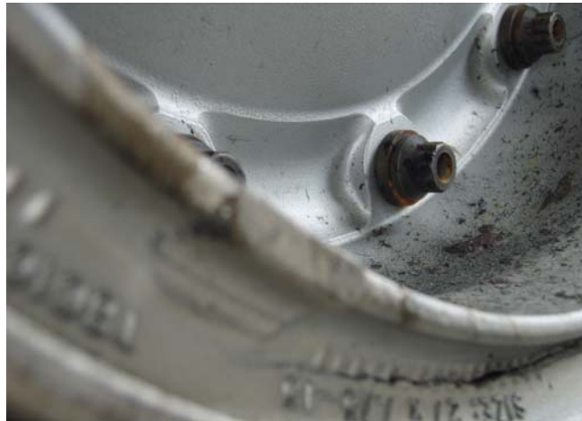
Figure 8: Wheel hub of the nose landing gear: crack
