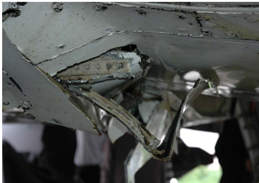
Figure 3: The Keel beam was broken
