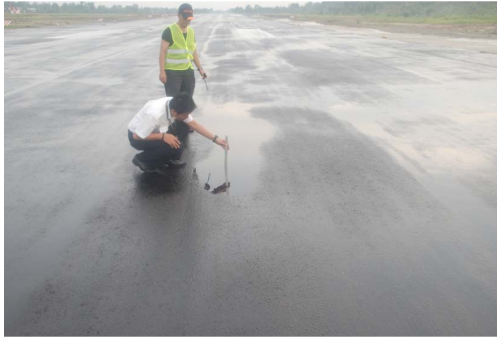
Figure 4: standing water examination performed 1 hour after rain.
