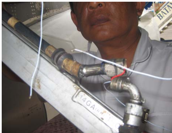
Figure 5: Broken left landing gear down lock cable
