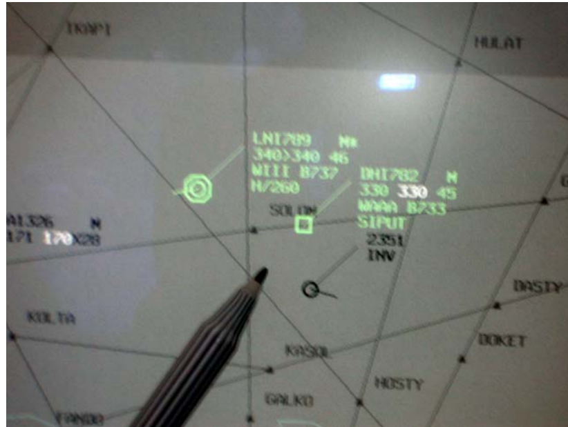
Figure 8: Flight plan track target (square with label, green color) was separated from radar track (circle with squawk number label, black color)
