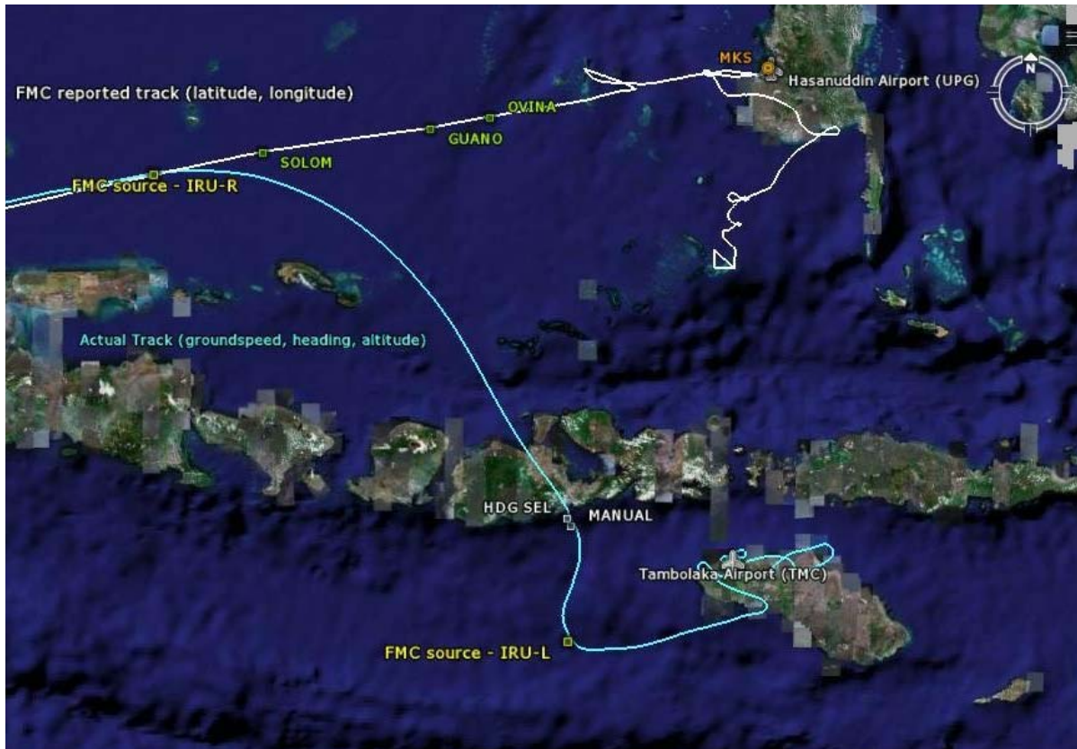
Figure 3 : Flight paths (FMC and actual) following switch to IRU - R
