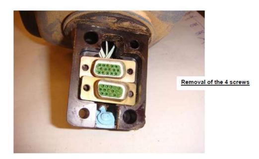
STEP12: A /P DISCONNECT AND PRIORITY SWITCH REMOVAL
