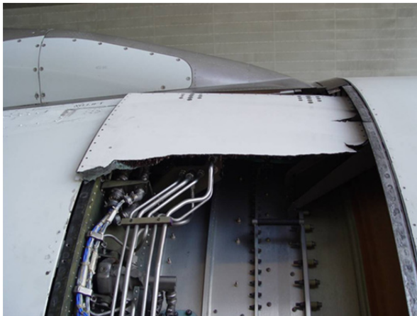
Residual fracture, right and left side
