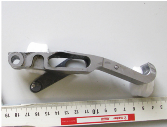
The approximate position of the link versus an undamaged latch
