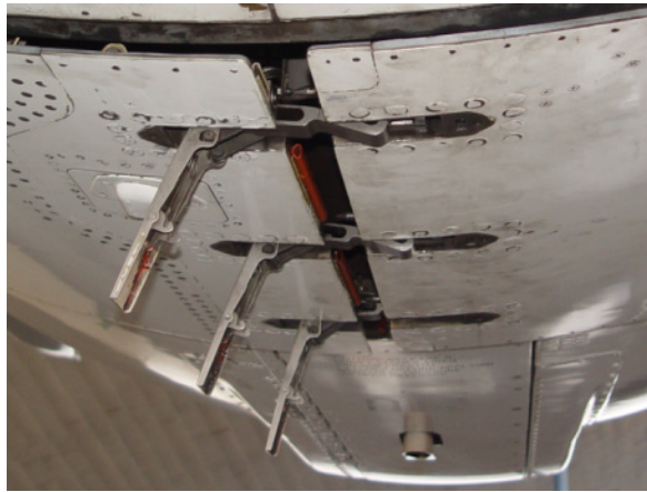
Closed cowling with one clasped latch (aft) Photos (2): BFU
