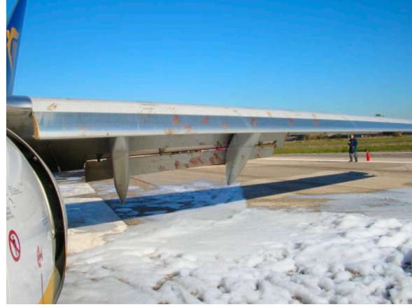
Photo 13 and Photo 14 : impact of birds on wings
