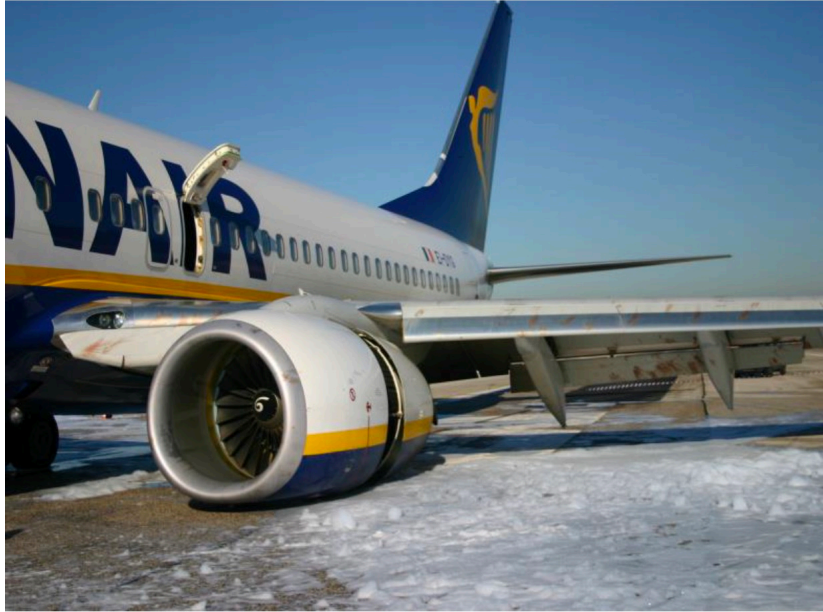
Photo 19 : thrust reverser locked in a partially opened position
