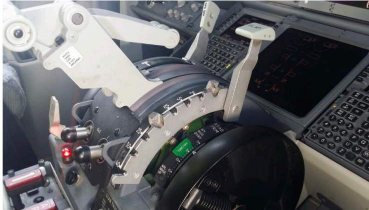
Photo 1: a flap control lever
