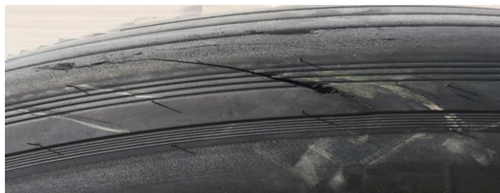
Figure 1. Damaged No. 3 main wheel tire
