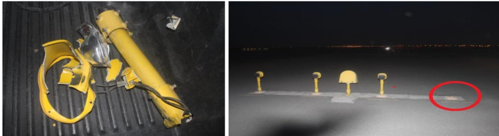
Figure 2. Damaged runway 30 approach light
