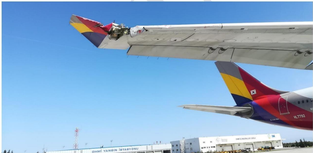
Picture-15: Damaged Right Wing of HL7792
